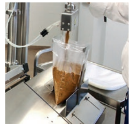
Dosing directly from kettle with pump
