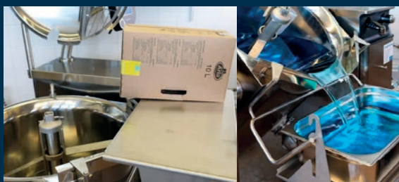
Pouring platform, works in two positions: for emptying the liquid pack and for emptying the kettle
