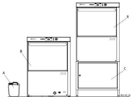
The detergent (A) is placed below the door's (B) bottom edge. If the machine is equipped with stand (C), the detergent can be placed there.
