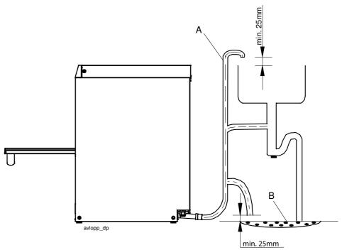
A=drain hose B=floor drain
