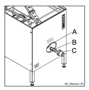
Removing/fitting the filter A=Filter housing B=Filter C=Cover
