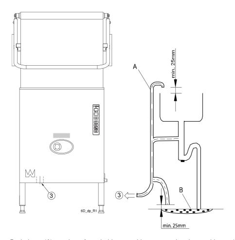
Drain hose (A) consists of a spiral hose and is connected to the machine at (3) and to the floor drain (B) as per one of the alternatives in the illustration.
