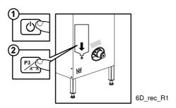
Note that emptying is necessary when you want to unscrew and clean the filter, because otherwise the water from the tank will spill out onto the floor.
