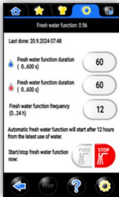
Fresh water function rinses the water pipes when the kettle has not been used for a certain time. The function rinses stagnant water and any deposits from the pipes. The Fresh Water Function page shows when the function was performed the last time.
