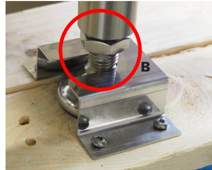
The kettle's transport base is equipped with brackets, to which the kettle is attached using the locking nuts of the leg on the frame (A).
