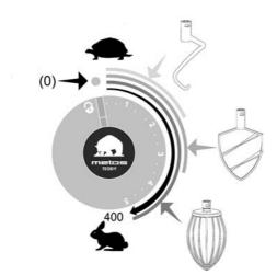
Fig 4. Recommended working speeds
