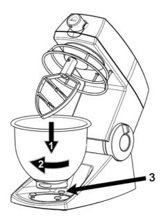
Fig 3. Placing the bowl on the mixer.
