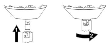
Fig 2. Mounting of the tool in the bayonet shaft
