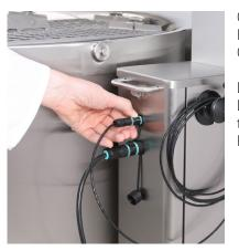
Connecting: Remove the cap from the socket. Connect the connector by pushing it into the socket.
