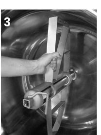
Make sure that the mixing tool is locked in its place by trying to lift/pull it out of its place by pulling at the mixer blade, for example.
