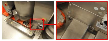
• Make sure the kettle is in position and the holes in the free standing frames of the kettles align.
