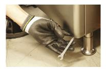
• Remove the cover plate of the left hand kettles control pillar (10 mm spanner).
