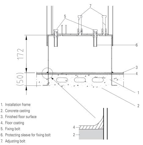
Place the kettle on the installation frame and adjust to a horizontal position with the adjusting bolts. When the kettle is in a horizontal position, it must be fixed to the installation frames with the help of the fixing bolts. The control pillar has 4 bolts and the support pillar has 2 bolts. Tighten the adjusting nuts carefully. Do not seal the space between the kettle pillars and installation frame as there must be enough change of air.
