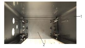
• Next, the control pillar (1) is adjusted by means of the adjusting bolts (3), to a horizontal position and on the same level with the support pillar. When the control pillar (1) is in position, it is fixed to the installation frame (2) with four fixing bolts (4). Check that the space between the kettle section and the support and control pillars is the same, both at the top and at the bottom.
