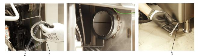
• Mount the locking ring (1) and secure it with the two locking screws (2) (4 mm Allen key). After that the cover plate of the kettles control pillar can be refitted (3) (10 mm spanner).
