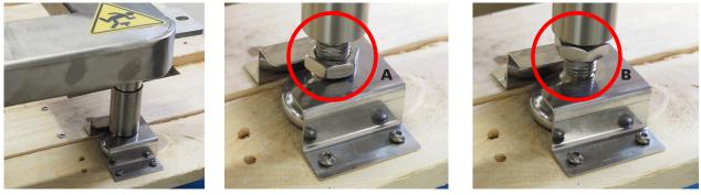
The kettle's transport base is equipped with brackets, to which the kettle is attached using the locking nuts of the leg on the frame (A).
