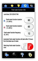
Fresh water function rinses the water pipes when the kettle has not been used for a certain time. The function rinses stagnant water and any deposits from the pipes. The Fresh Water Function page shows when the function was performed the last time.
