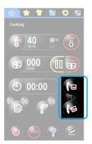
This option enables forced mixing at the lowest mixing speed while the kettle is tilted. With the help of this function it is possible to portion more homogeneous batches of food into smaller bowls.
