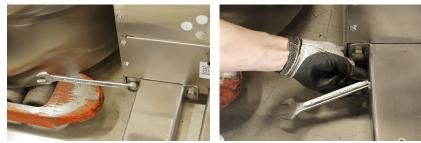
• Fix the kettles together with four 12 mm bolts using the 19 mm spanner.
