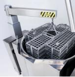
Integrated lifting arm capacity is 200 kg.
