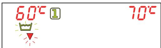
**Salt level warning (option).** When the **F8** indicator flashes on the display it means that the salt level in the bowl is low (only on machines equipped with the optional Water Softener).
