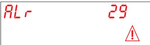
**Z9 REGENERATION FAILED (on machines equipped with the optional Water Softener):**
