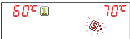
**Detergent level warning (option).** When the **F10** indicator flashes on the display it means that the detergent is over (only on machines equipped with the optional "Chemicals level Sensor").
