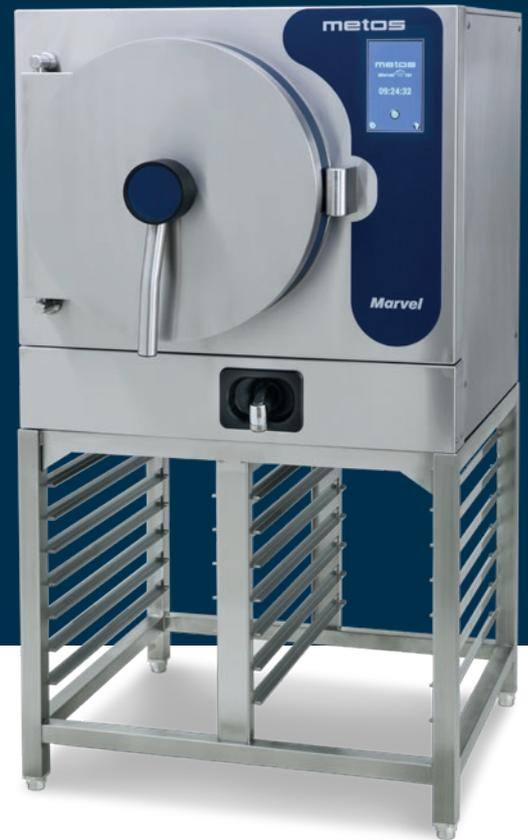
Metos Marvel Pressure Steamer cooks, defrosts and regenerates all types of food products, including delicate items. Thanks to its dedicated steam generators, the Metos Marvel can steam at user defined temperatures up to 120°C (1bar). The Metos Marvel has a chamber of acid proof stainless steel, allowing to cook 4x GN 1/1 65 mm or 3x GN 1/1 100mm pans. A core temperature probe for delta T cooking or sous vide products is an option.
