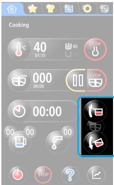
This option enables forced mixing at the lowest mixing speed while the kettle is tilted. With the help of this function it is possible to portion more homogeneous batches of food into smaller bowls.
