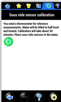
The Sous Vide sensors (Sous Vide sensor rod and the product core temperature sensor) calibration page appears on the screen.
