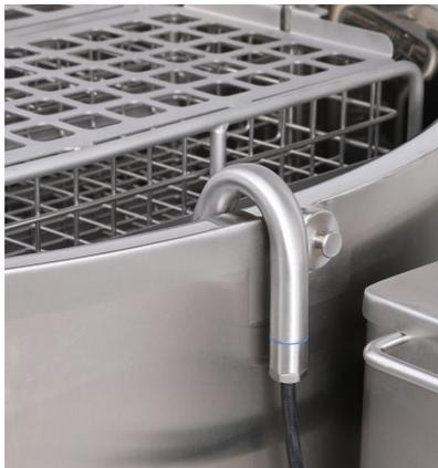
Place the Sous Vide sensor rod in the kettle so that its stem is just behind the hanging peg of the safety grid.
