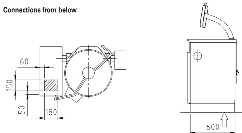
2. Cold water connection R1/2" (  $\phi 15$  ). Must be fitted with a one way valve and shut off valve.
