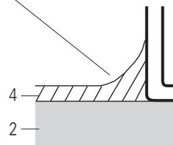
Place the kettle on the surface installation frame and adjust to a horizontal position with 4 adjusting bolts. When the kettle is in a horizontal position it must be fixed to the surface frame with the help of the fixing bolts. The control pillar has 4 bolts and the support pillar has 2 bolts. Tighten the fixing bolts carefully. Do not seal the space between the kettle pillars and surface installation frames, as there must be enough change of air.
