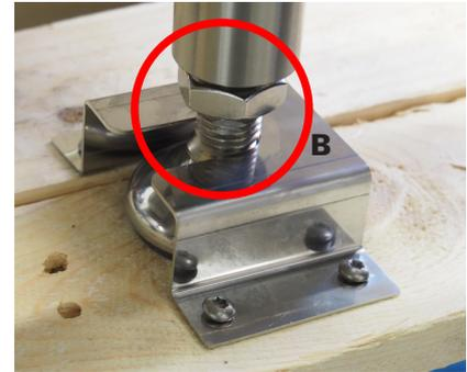
The kettle's transport base is equipped with brackets, to which the kettle is attached using the locking nuts of the leg on the frame (A).
