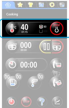
**i** Cooling is only switched on when the kettle is in upright position (cooking position). If the heating function is selected when the kettle is not in upright position, the message “Kettle not in cooking position” appears on the display
