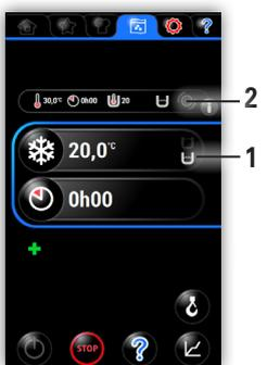
The order of the phases can be changed by activating the desired phase by holding it down and dragging it to the desired position.
