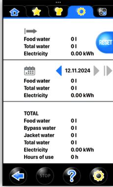
This function allows you to check the electricity (electrically heated kettle) and water use. The function does not measure the water used with the hand-held shower.
