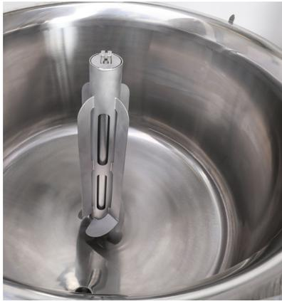
Install the Sous Vide circulator by placing it in its place in the kettle.
