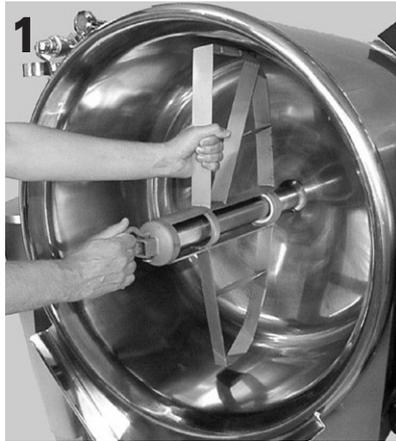
It is easiest to attach the mixing tool to the mixer axle when the kettle is in a tilted position. Push the ring on the mixing tool into the kettle's mixer axle and fit the mixing tool in place, while the lifting handle is straight so that the locking device of the lifting handle sets in the groove at the upper end of the mixer axle.
