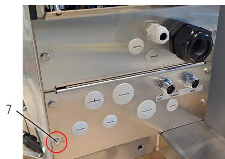
Detach the lead-through plate (2) from the pillar. Slip the supply cable (1) through the cable bushing (3) of the lead-through plate. Connect the phase wires of the cable to the mains switch (4) and PE and N cables (5, 6) to the terminal blocks.
