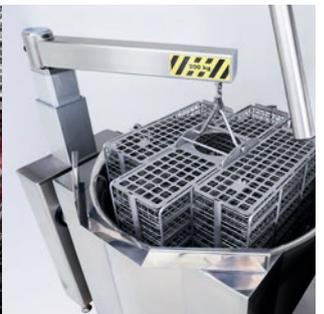
Integrated lifting arm capacity is 200 kg.
