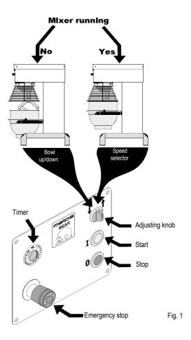
The operation panel is provided with an adjusting knob with two functions (fig.1):
