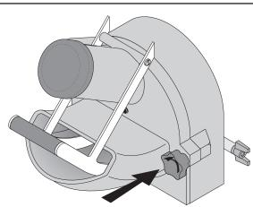
When cleaning the vegetable cutter or when the cutting disc is to be exchanged, open the front part by turning the thumbscrew counter-clockwise. For safety reasons the cutting disc stands still when the front part is opened.
