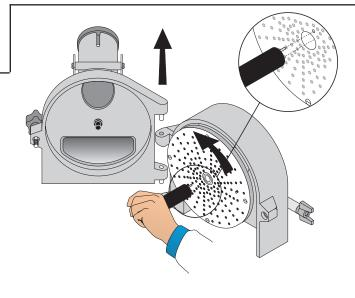
When the front part is open, it can be lifted off in order to make cleaning easier.
