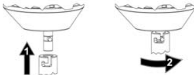
Fig 2. Mounting of the tool in the bayonet shaft
