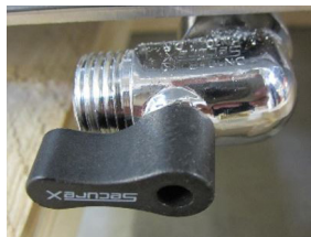
1. Control valve of steam generator
