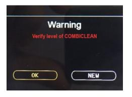
If the cartridge is empty, replace it following the instructions in the following paragraph, otherwise confirm the "OK" message by pressing knob **16** to start the wash.
