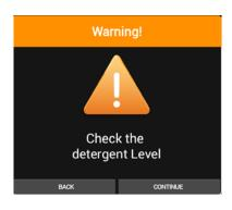
If the cartridge/canister is empty, press "BACK" **(4)** and replace it by following the instructions in the paragraph "REPLACING THE DETERGENT/DESCALER CARTRIDGE" **(5)** before starting the wash cycle.
