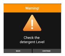
If there is not enough detergent to run the selected wash cycle, a popup window will appear on the display telling you to visually check the detergent/descaler level (1).
