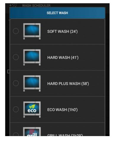
Select the desired wash cycle and confirm by pressing **OK**.
