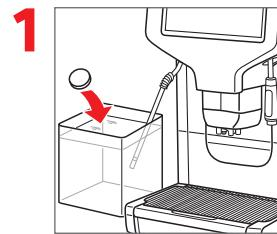
Submerge steam wand / iSteam in milk cleaning solution
