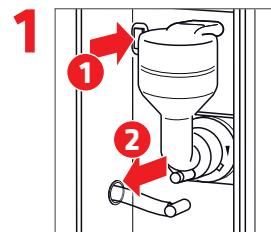
Open front door, switch off, remove tube
