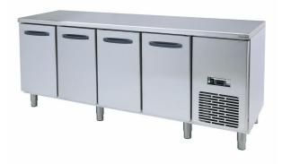
the device from getting dirty. The device has an automatic defrosting and evaporation of the meltwater, as well as a standard drainage possibility. Door gasket can be replaced without any tools. The cool cabinet is supplied with connectors for power cables at the bottom of the device, making it easier to keep the floor under the device clean.
