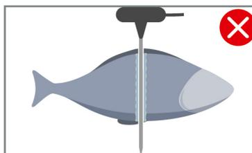
1. Insert the core probe up to the handle into the thickest point of the food.
