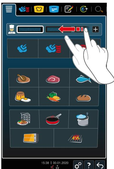
>> When you open the start screen, the activated profile is displayed. If several profiles are displayed, you can scroll through the list. To Create a new profile [▶ 77], press the button: +
