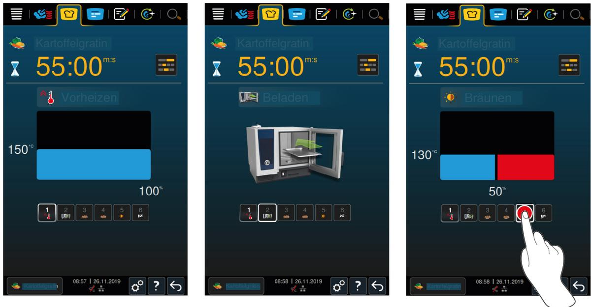
If you have started an intelligent cooking path, the display changes to the cockpit after a short time. All cooking steps that the intelligent cooking path processes are displayed here one after the other. The active cooking step is highlighted. The cooking steps that will take place in the future are greyed out. When the cooking step is completed, the next cooking step is automatically displayed.
