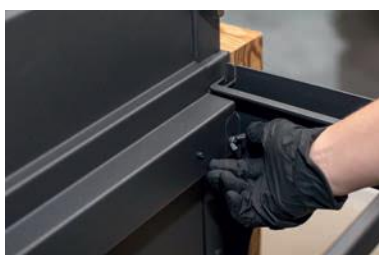
Undo the wing screw on the right side and remove the bracket that becomes free.
