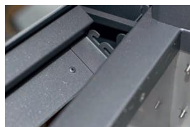
Then pull the mirror off the guide pin on the left side.
