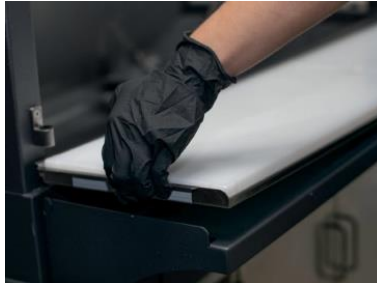
Lift the chopping board attachment out of the fixture.
