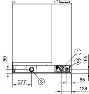
① Electrical connection: Semifixed, 2,5 m cable without plug
