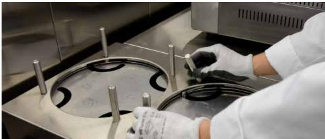
Remove the rods by screwing them counter-clockwise
