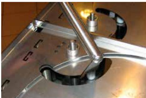
Slide the adjustment rods (4 pcs/cylinder) in place. You do not need to remove the cylinder from the appliance..
