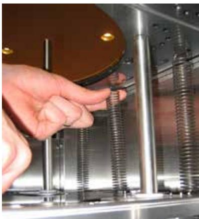
Attach the spring into the slot in the cover.
