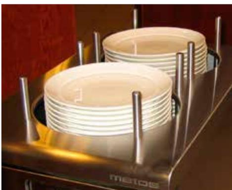
Detach the dispenser cover by untwisting the support rods (4 pcs/ cylinder) which hold the cover in place.
