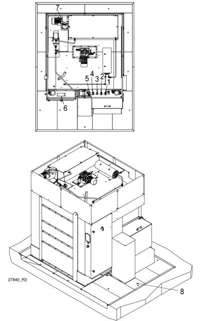
The machine is installed "recessed into the floor"
