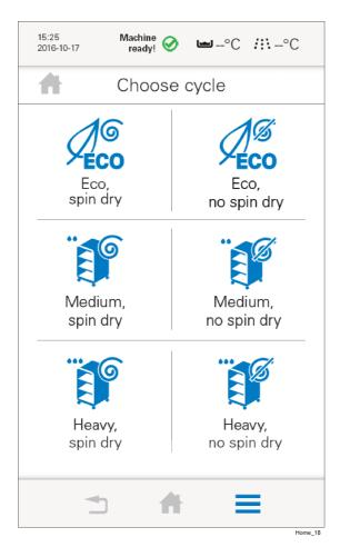
When the machine is ready to starting washing, the following display is shown on the touch panel.
